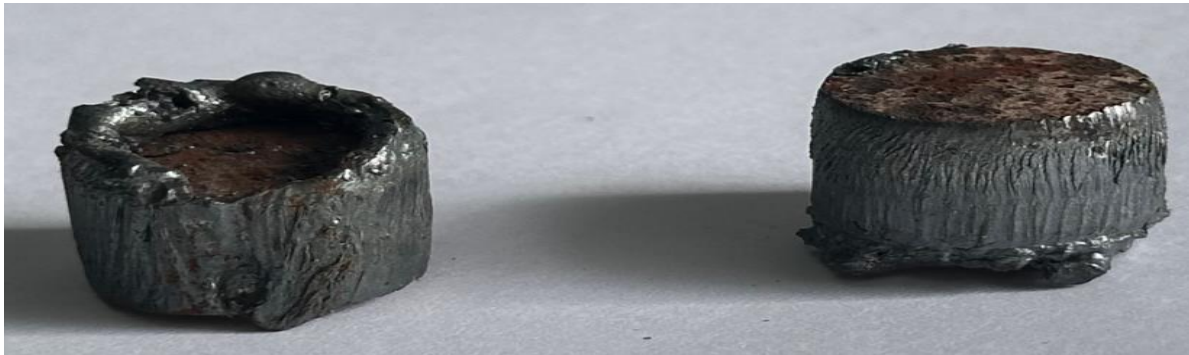
Figure 1. Macrostructure of the edge surface after laser cutting.
